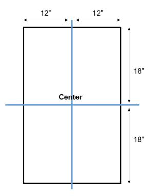
After finding the center trace out the edges of the shield, making sure all four quadrants are equal in size and shape. Here is an example outline for a 24" by 36" oval shield:
